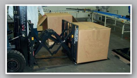
Ekosheet® represents a range of high quality plastic sheets for material handling, storage and transport. These PE or PP based products are used as a slipsheet or separation sheet. Ekosheet® can be handled with Push-Pull or Rollerforks® equipment.
